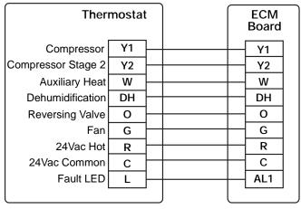
Units with CXM or DXM board and ECM fan motor, utilizing ECM dehumidification mode
